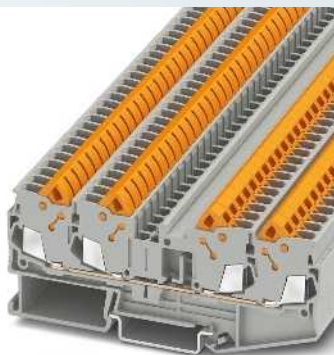
2.5 (2.5) mm 2 , 24 A, feed-through terminal block, four connections
