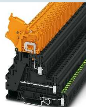
4 (6) mm², 36 A, multi-level terminal block, disconnect lever, PE foot
