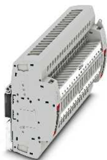
6 (10) mm², 30 A, test terminal strip, for DIN rail mounting, VDE coded type B19
